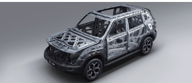
Ultra-Safe Cage Body Structure with Integrated Laser Tailoring
